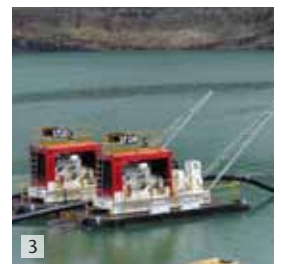
1: Single and double electric pontoon pump units
