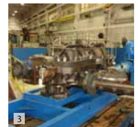
3: Testing a high pressure multistage slurry pump
