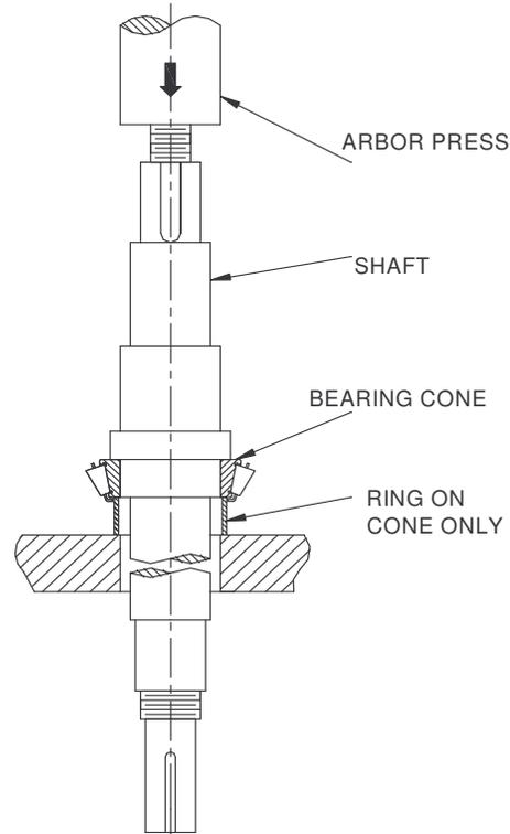
Heat the bearing in an oil bath or electric oven to a uniform temperature of 120 °C (250 °F). When heated, quickly mount it on the shaft. If the alternate method is used, apply force by means of an arbor press; see detail below. Use a tubular sleeve, ring, or small blocks of equal thickness to apply the force to the cone (inner race). In forcing a bearing onto a shaft, be careful that the cone is never cocked.
