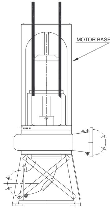
c) MF pumps that are < 135kg (300lb.) Eye bolt lifting- without the fabricated stand.
