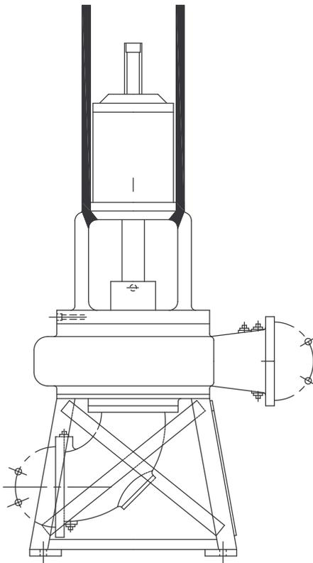
b) MF pump + stand+ motor base- lifting (all sizes)
