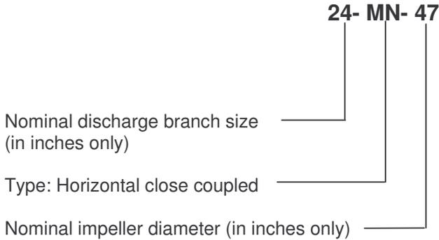
**Note:** Measurement shown above for discharge branch size and impeller diameter are always provided in inches.
